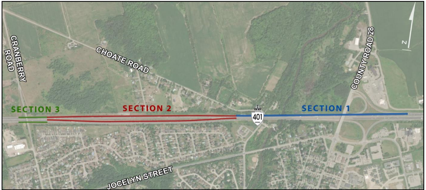
Figure 42 – Recommended Highway 401 8-Lane Footprint
